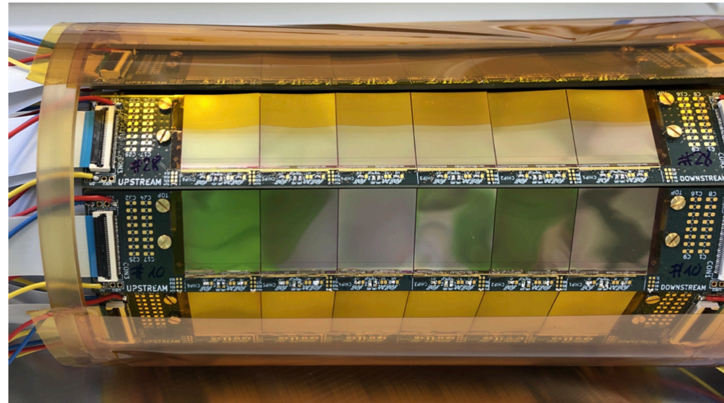
Vertex detector prototype with MuPix10 chips for Mu3e
