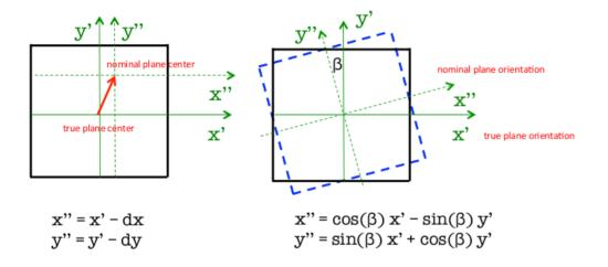
→ Several iteration after each correction (order of 200) to reach stability in results → determination of offsets and rotation around beam axis
