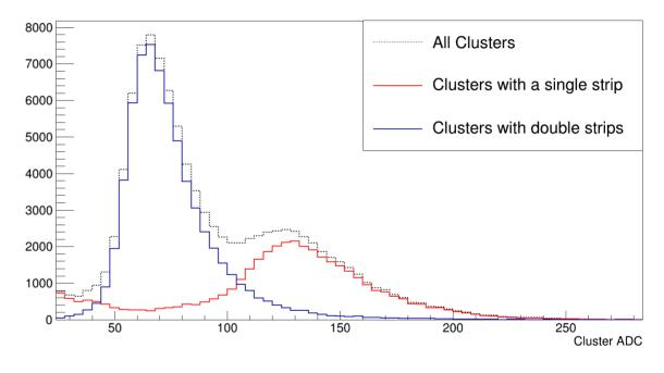
→ dE/dx distribution as a function of proton position among two readout strips for 70 MeV protons.
