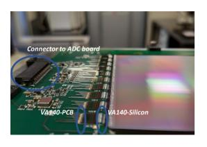
MSD is the Silicon Strip Detector after the magnets, for measuring the charged fragment positions (momentum) and their dE/dx.
