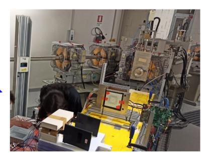
Once we inclined the sensors to study the passage of protons through several strips to measure dE/dx distribution.
