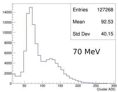
Two peaks response is due to the floating strips configuration chosen: 1 over 3 strip readout.  $\rightarrow$  different CCE according to position
