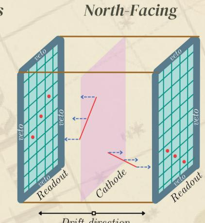
Recoil imaging detectors using Micro Pattern Gas Detectors (MPGDs) will be highly segmented in one plane, so it is
