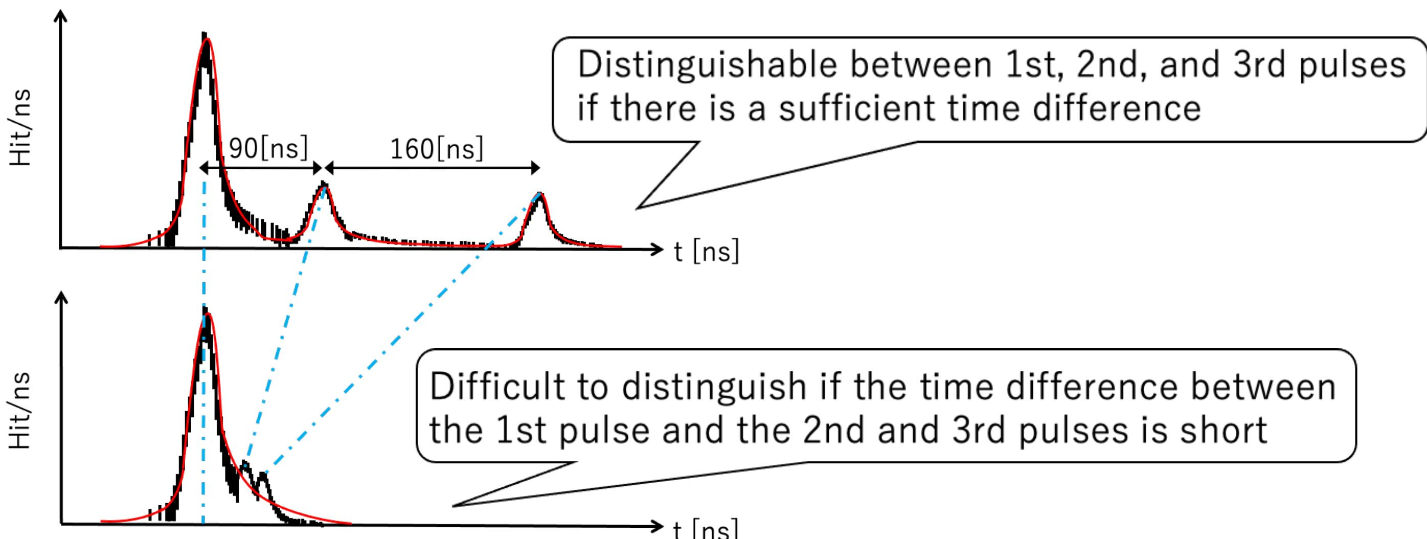
Distinguish waveforms from  $\chi^2$  obtained by fitting
