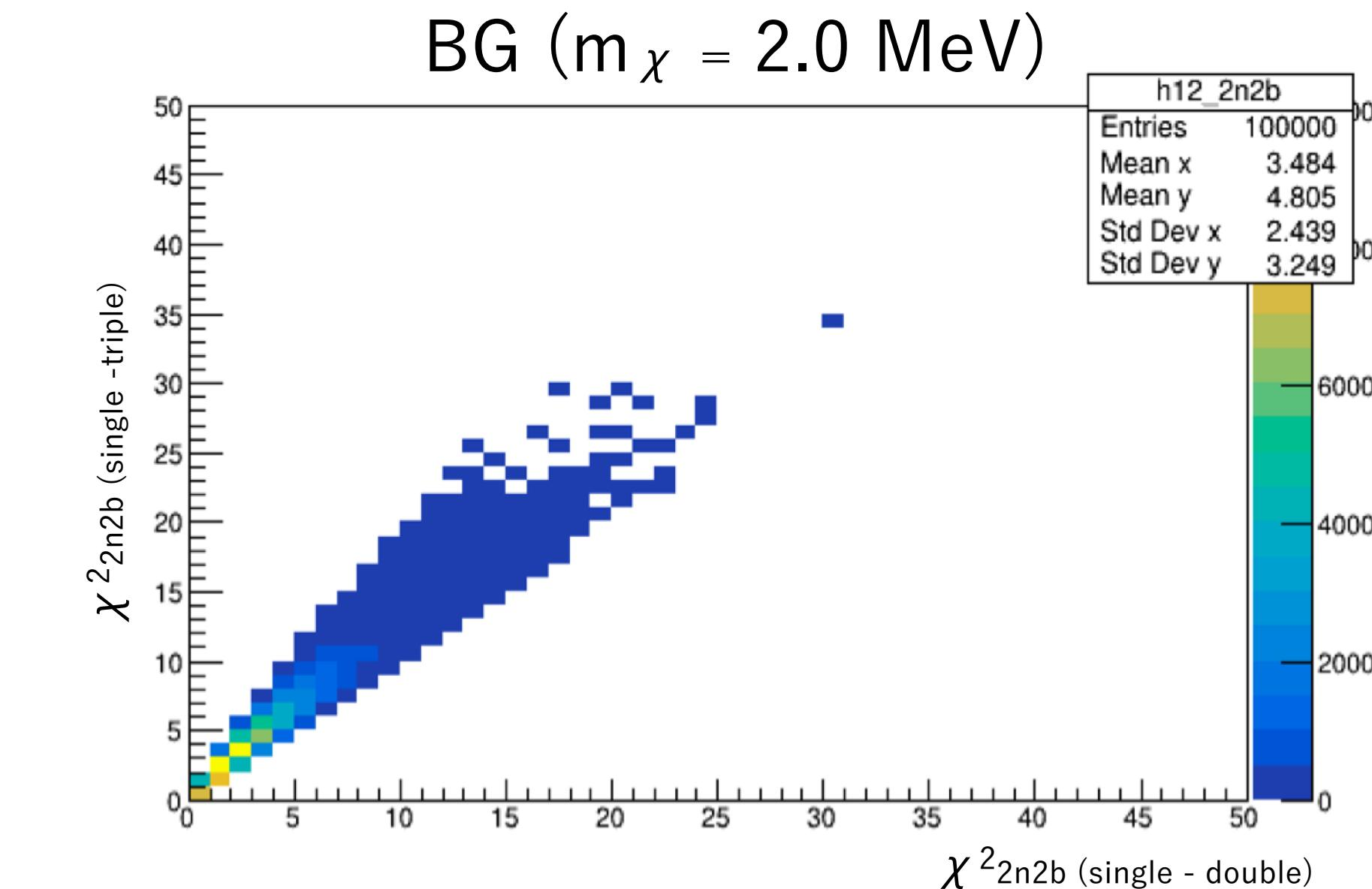
→  $\chi^2_{\text{single - triple}}$  makes it easier to determine whether single or multi pulse
