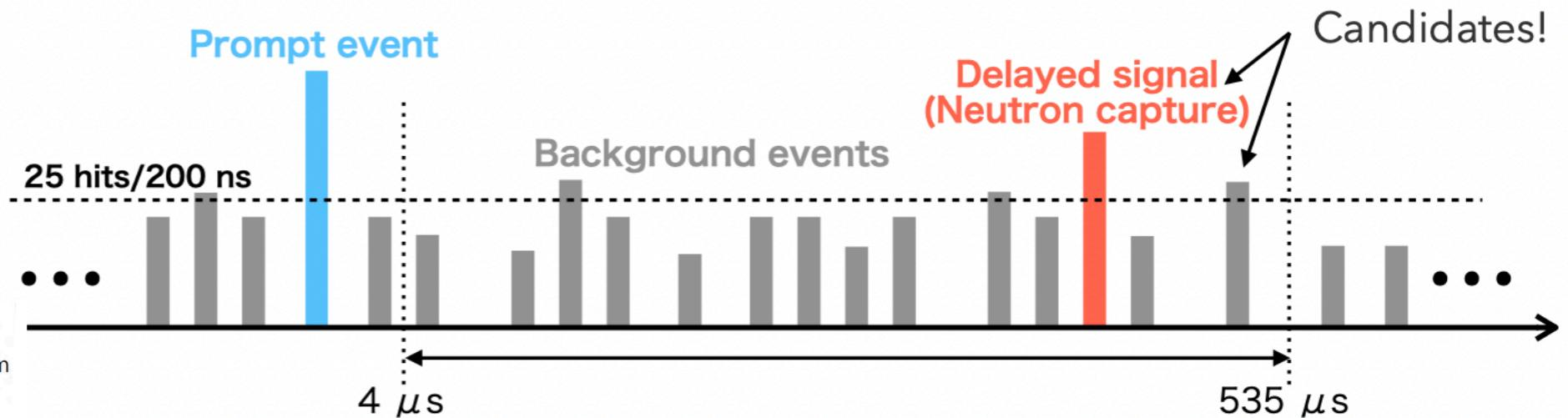
When SHE trigger is issued without an OD trigger, **AFT trigger** is issued → all hits in the 535  $\mu$ sec recorded for neutron tagging (reduce BG)
