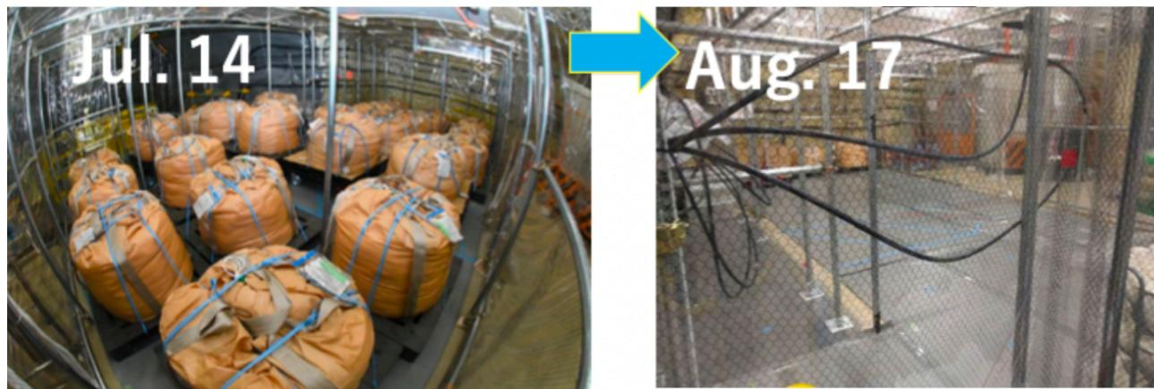
The 2nd Gd-loading Jun. 1 - Jul. 5, 2022 (35 days to replace 50,000 tons of 0.01% Gd water with 0.06% Gd water at 60 m<sup>3</sup>/h) → start of SK-VII !
