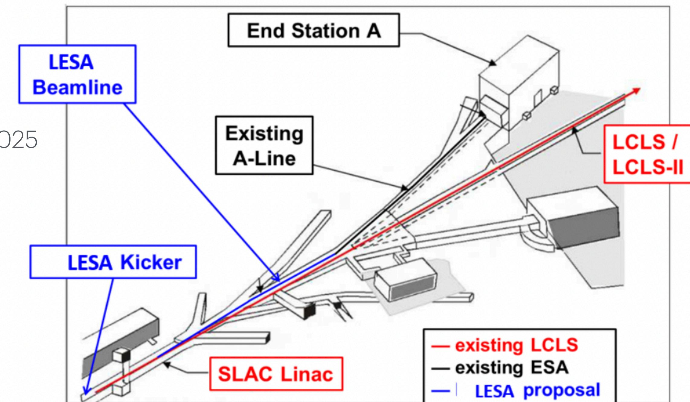
Beam layout, from The SLAC Linac to ESA (LESA) Beamlne for Dark Sector Searches and Test Beams [[arxiv:2205.13215](https://arxiv.org/abs/2205.13215)]
