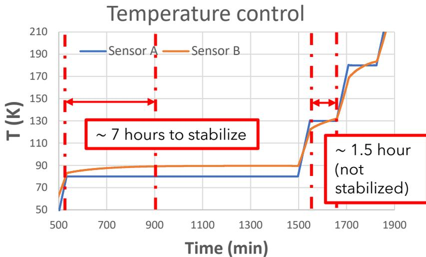
The stabilization of Sensor B temperature takes several hours (depending on the temperature). More time is needed for the correct stabilization of the bulk crystal.
