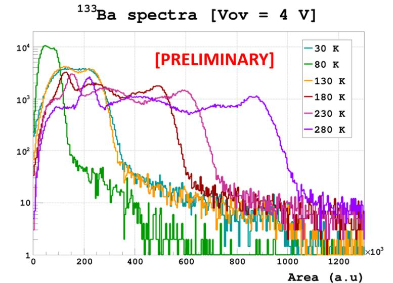
We observed the loss of LC when lowering the T. Possible contributions of the reduction of LY in NaI(Tl) and the emission spectra shifting to wavelengths where the SiPMs are less sensitive.
