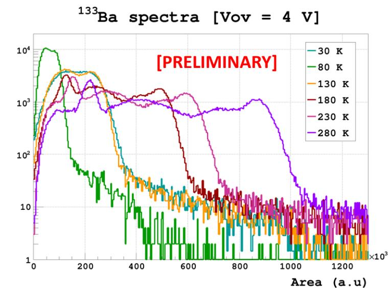
We observed the loss of LC when lowering the T. Possible contributions of the reduction of LY in NaI(Tl) and the emission spectra shifting to wavelengths where the SiPMs are less sensitive.
