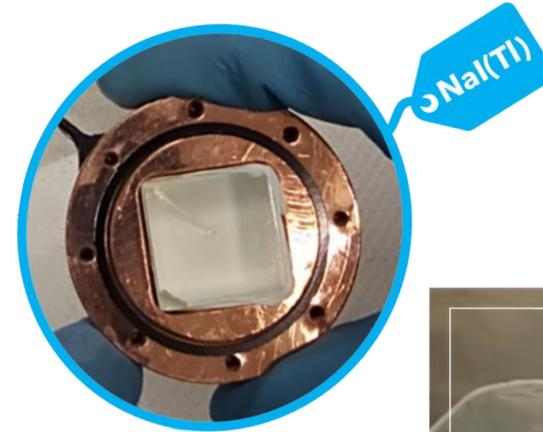
The crystals are stored and manipulated inside a dedicated glove box with low humidity atmosphere (filled with nitrogen gas).
