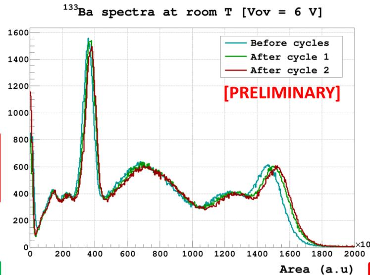
The first crystal tested in two thermal cycles seems to be undamaged.
