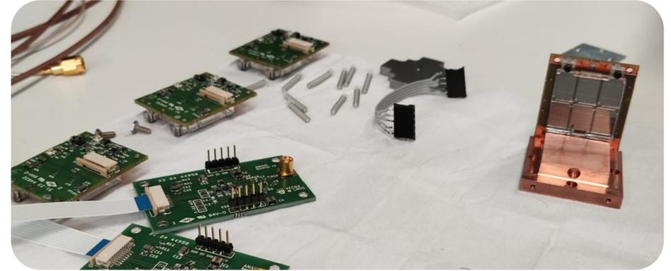
SiPMs and electronics developed at LNGS.
