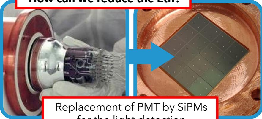
Replacement of PMT by SiPMs for the light detection
