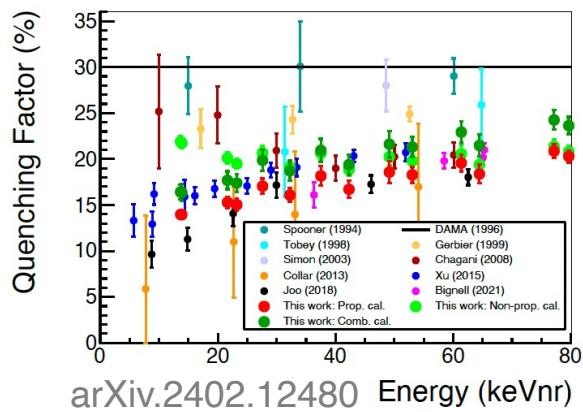
nPR measurement for COSINE-100 crystals
