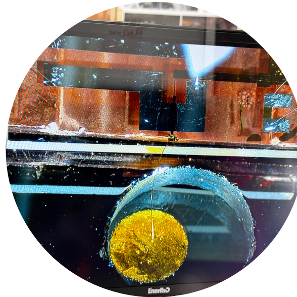
Si-beaker for 4\pi active surrounding of the crystal
