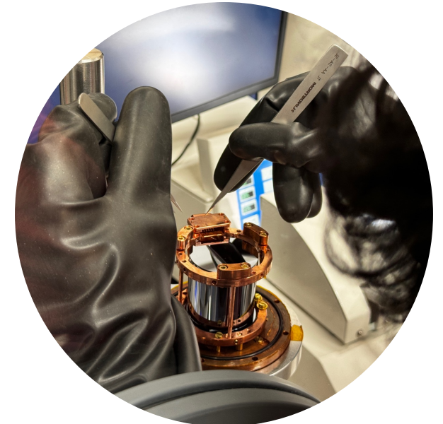
Si-beaker for 4\pi active surrounding of the crystal
