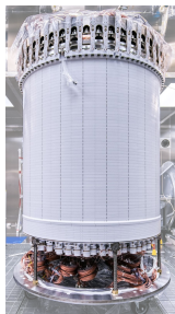
TPC assembled and moved underground
