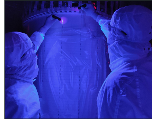
Dust inspection of the TPC with UV light
