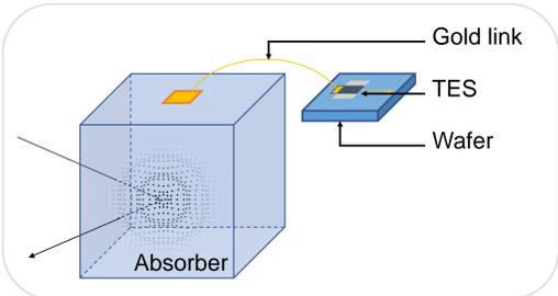
In the remoTES design the TES is not deposited directly on the absorber, but located on a separate wafer disk. A gold link consisting of a gold film and a gold bond wire connects the TES with the absorber. The benefits of this design are a wider choice of absorber materials, higher reproducibility and higher purity standards
