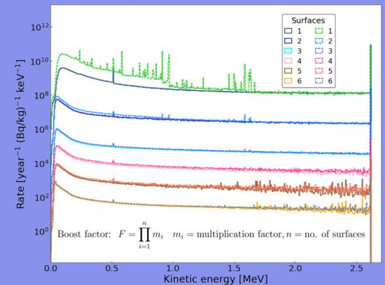
Figure 2: Gamma-ray energy spectra from  $^{208}\text{Tl}$  (solid line) and  $^{232}\text{Th}$  (dashed line) at each surface from the outside of the water tank and in stages throughout until reaching the TPC. By the time the  $\gamma$ -rays reach the TPC, only those originating from the  $^{208}\text{Tl}$  decay survive.
