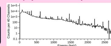
Figure 6. Left: A sample on Chaloner, a HPGe detector. Right: Example energy spectrum of a rock sample as measured by Chaloner.
