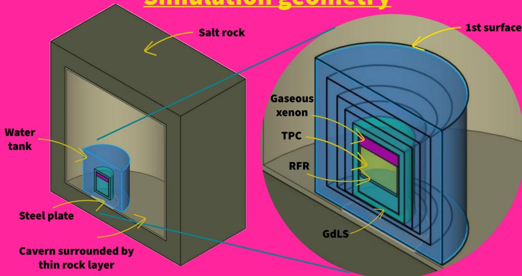
Figure 1: The GEANT4 [1] simulation generates  $\gamma$ -rays in a 0.5 m thick layer of rock surrounding a large, cylindrical cavern and transports them towards the TPC. They are stopped at each of the concentric surfaces before being propagated again towards the next surface in increased numbers.
