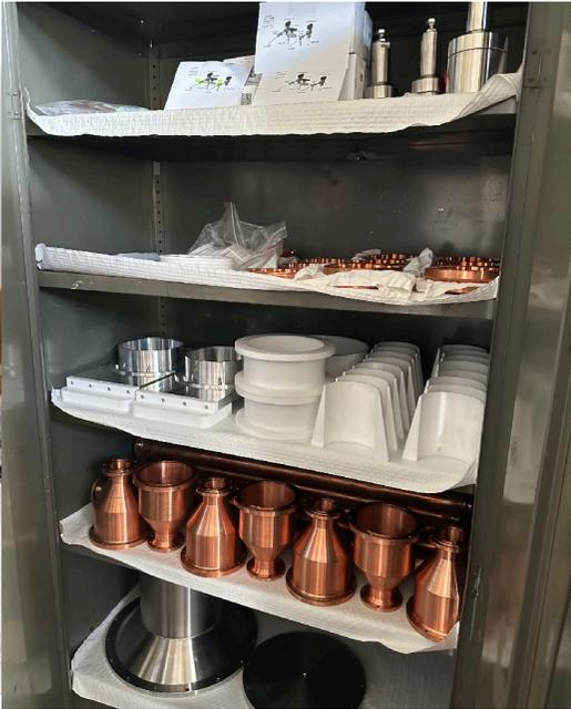
Crystals encapsulated in copper/PTFE enclosures, directly coupled to two R11065 PMTs. Purged with high purity dry N<sub>2</sub>.
