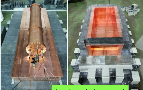
Lead castle for crystal assembly testing (pictured LNGS)
