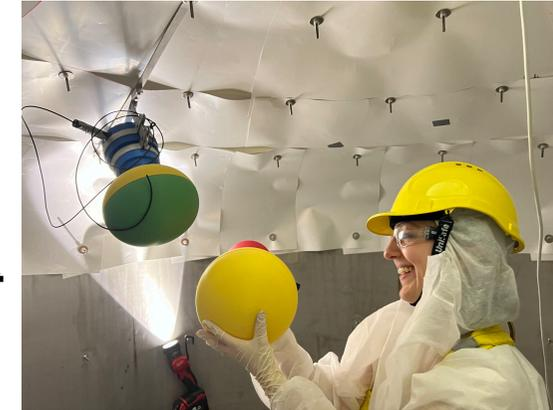
Veto vessel: Lumitor and PMTs installation tests
