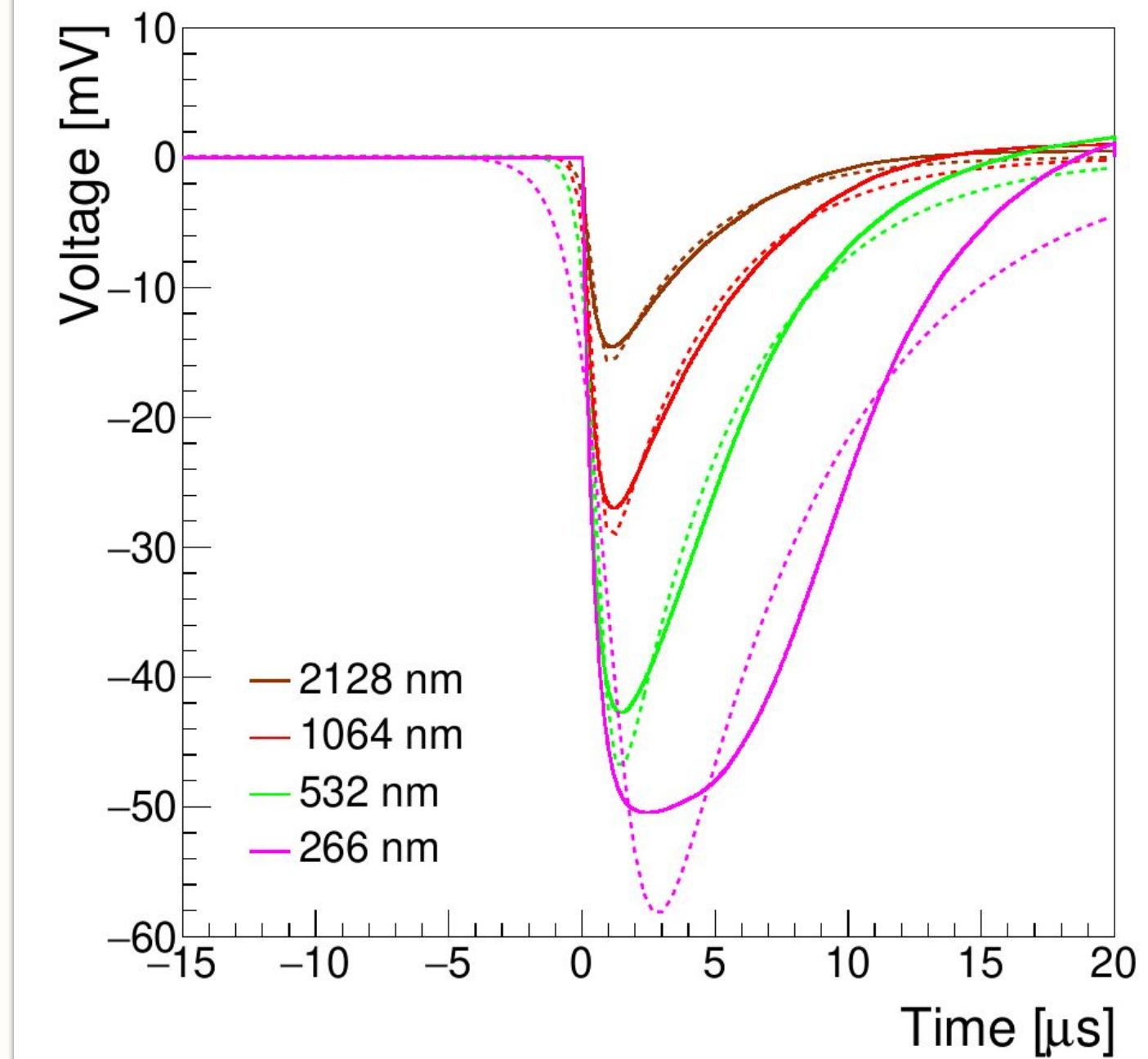
Simulated pulses of different wavelengths with fits
