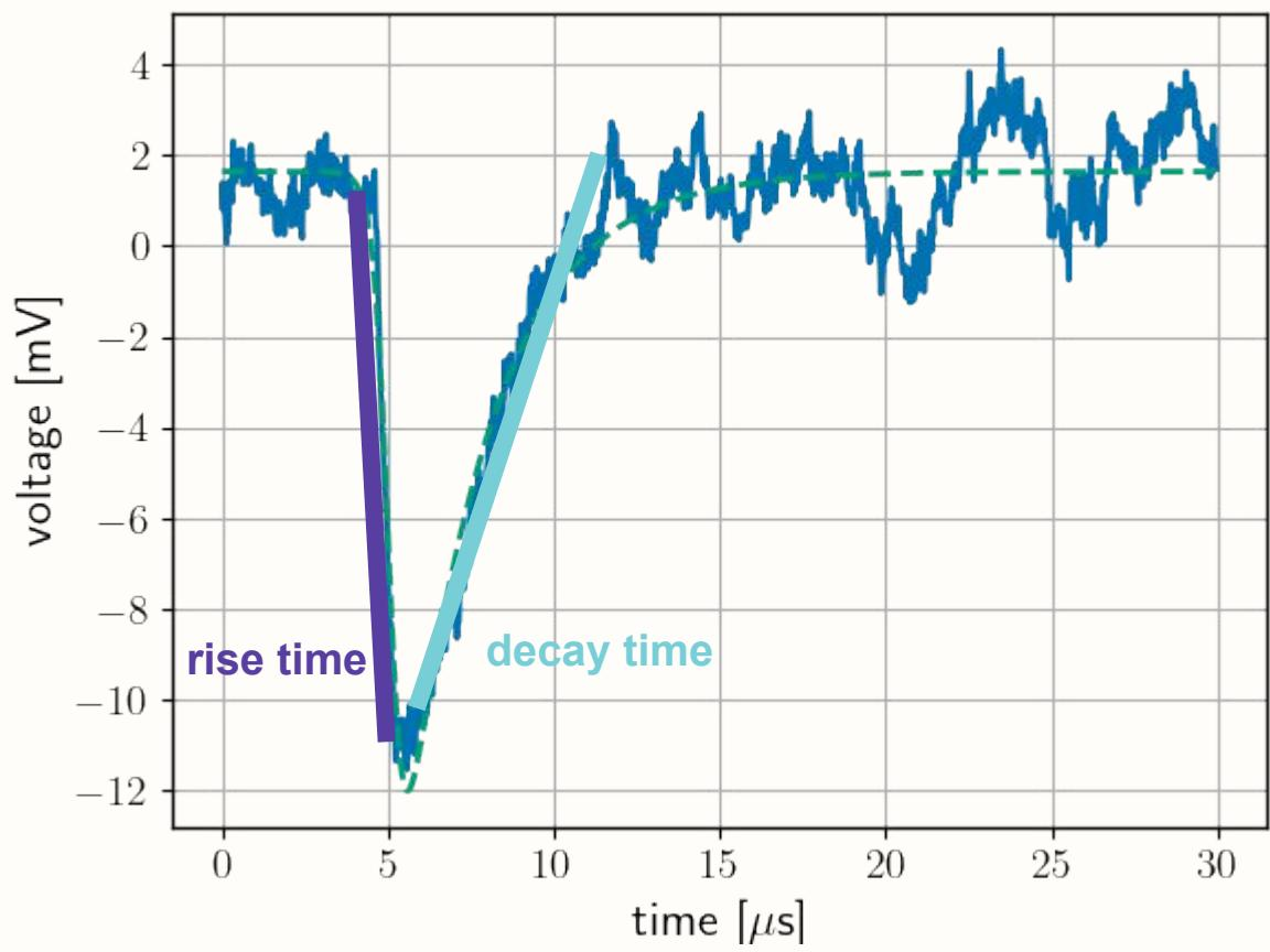
$$U(t) = -\frac{2A}{e^{-\frac{1}{\tau_{\text{rise}}}(t-t_0)} + e^{\frac{1}{\tau_{\text{decay}}}(t-t_0)}} + V_0$$
