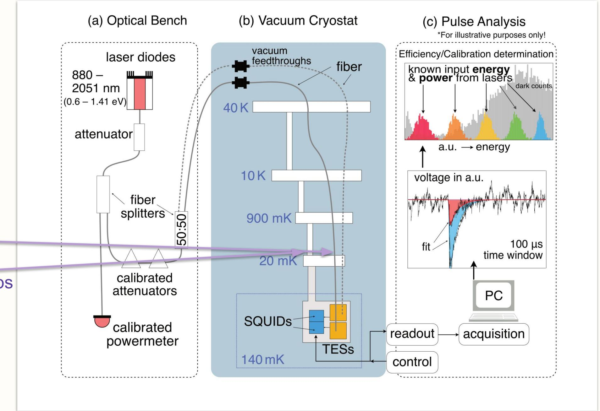
To mimic an intrinsic measurement, the fibers are placed on top of the 20 mK stage above the TES module to reduce black body radiation from the warmer parts of the cryostat. The light can enter the TES space through a small slit.
