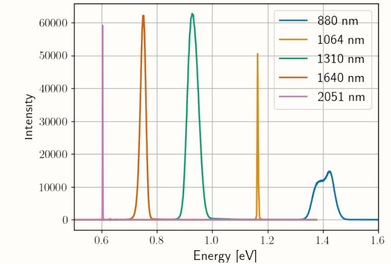
Energy spectrum of used laser diodes
