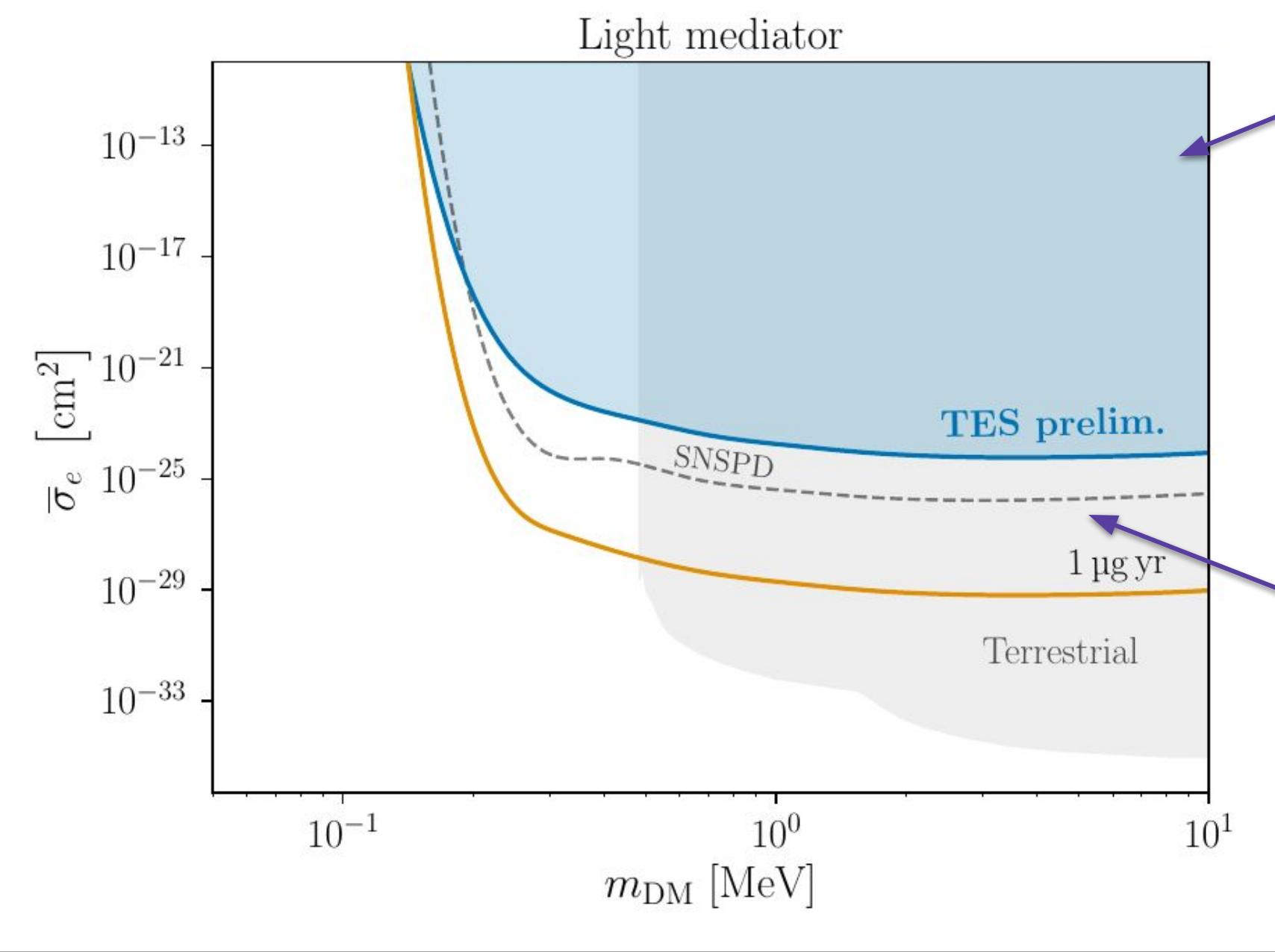
Possible sensitivity based on our TES setup (based on previous intrinsic measurements)
