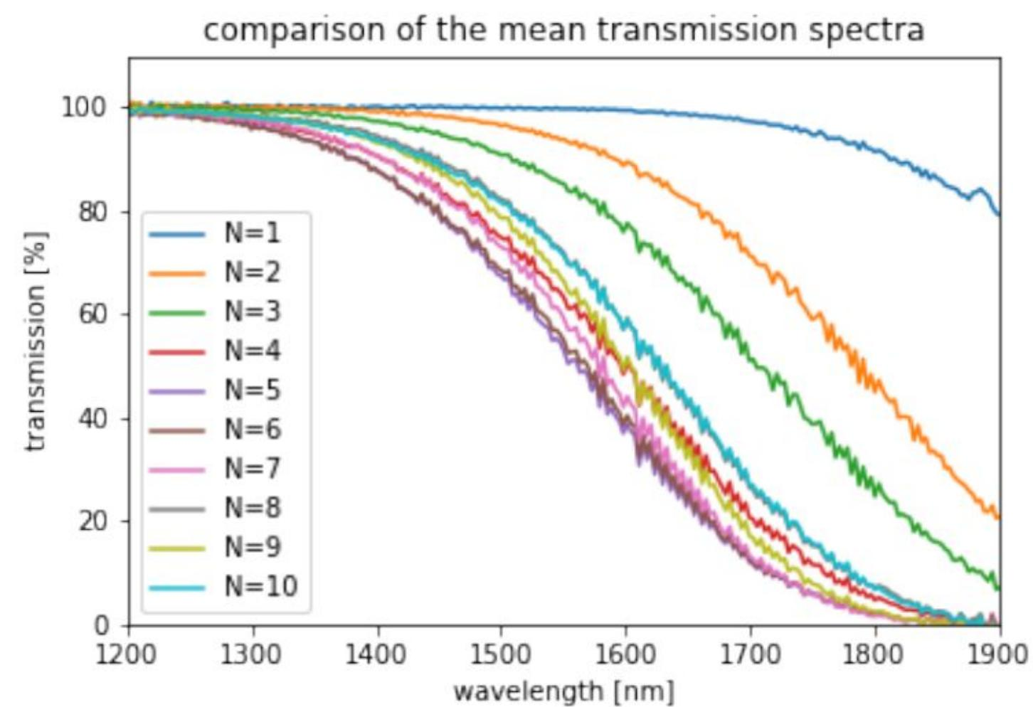
Transmission spectrum of a white light source for different windings of curled fiber - measured by intern Maria T. Pabst
