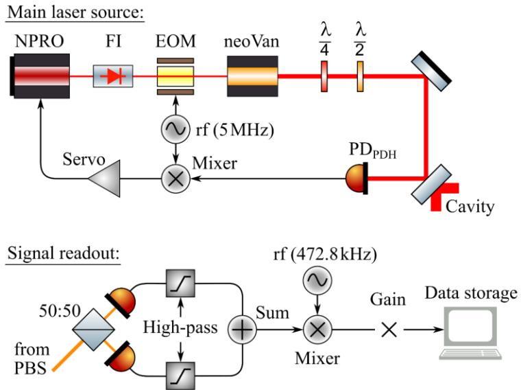
EOM: electro-optic modulator, NPRO: non-planar ring oscillator, PBS: polarising beamsplitter, PD: photodetector, PDH: Pound-Drever-Hall, rf: radio-frequency generator
