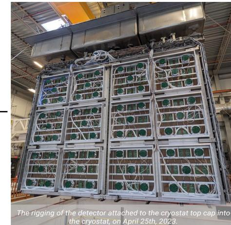
The rigging of the detector attached to the cryostat top cap into the cryostat, on April 25th, 2023.
