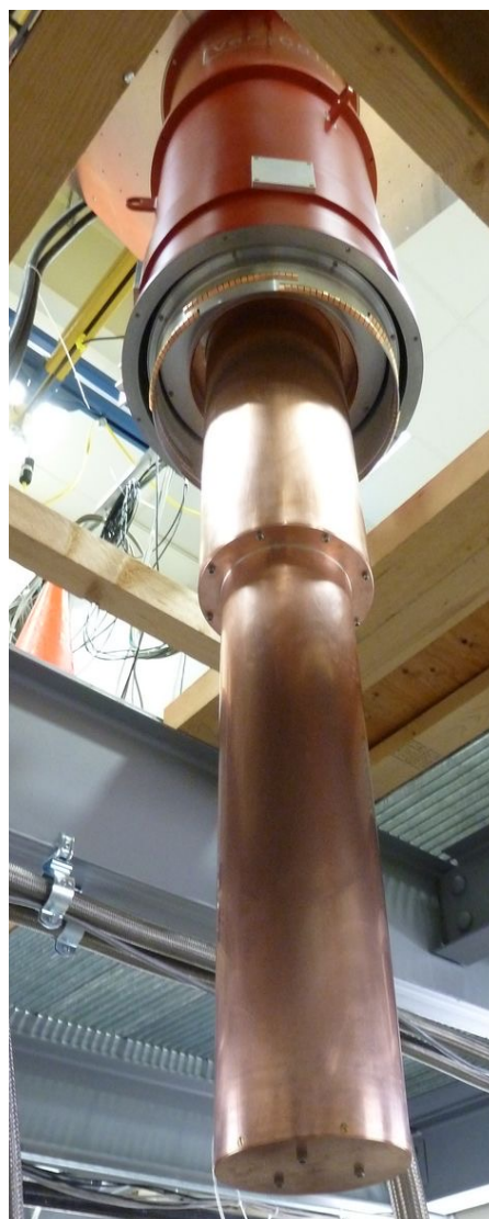
^3\text{He}/^4\text{He} Dilution Refrigerator
