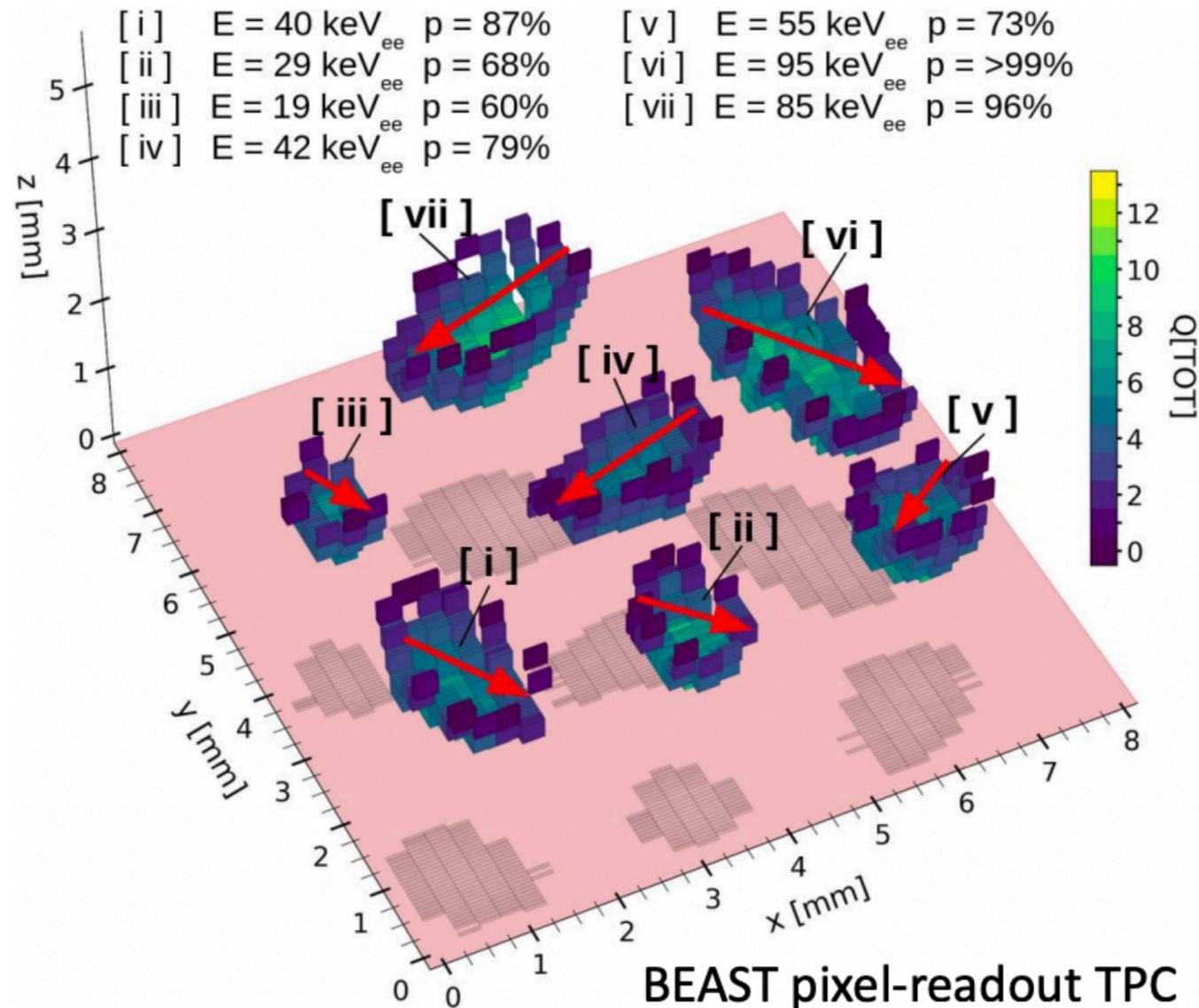
3D Pixel readout: event-level Head-Tail recognition on He recoils enabled through CNN (Schueler, Vahsen)
