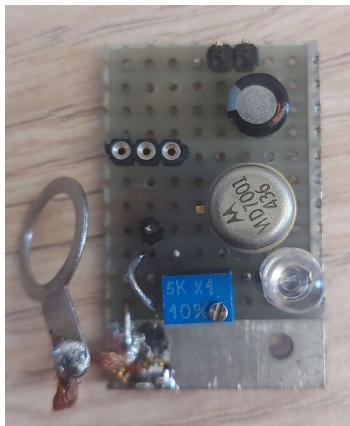
Single LED driver prototype with several circuit attempts
