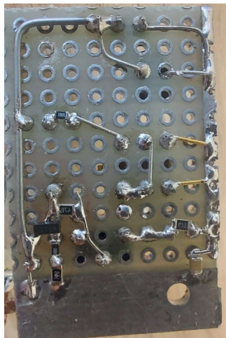
Single LED driver prototype with several circuit attempts
