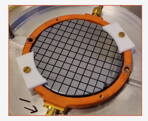
Obtain a cryogenic, **low threshold nuclear recoil detector** for light dark matter ( $0.1 \div 10$  GeV) searches and neutrino physics (CEvNS).
