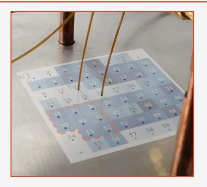
8 optical fibers firing on the diced side of the detector
