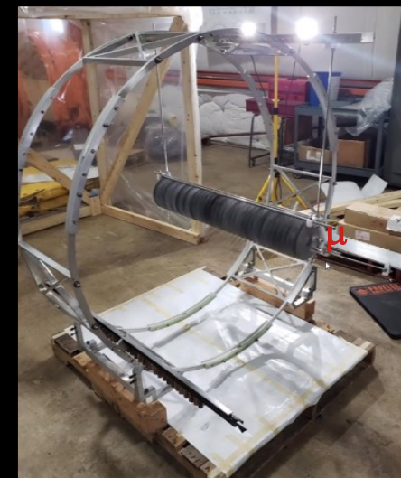
The Aluminum muon stopping target
