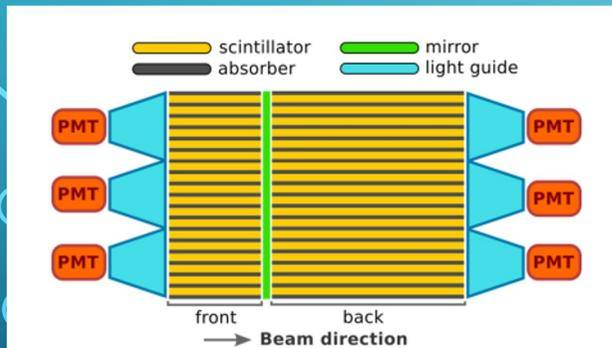
**SPACAL modules with Pb absorber and organic fibers (near the inner region)**
