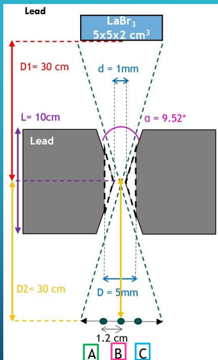
Preliminary MC simulations performed to estimate imaging capabilities of a Gamma camera based on square LaBr<sub>3</sub>:
