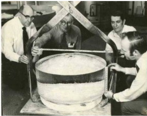
The first 32 inch diameter NaI(Tl) crystal. Pictured from left to right are Dr. Swinehart, Ed Jablon, Joe Kraus and Marko Stigoi.
