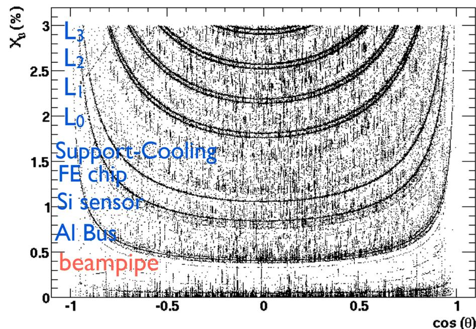
*Total SVT material is about 3.3% (2.4%)  $X_0$  for  $L_0$  Hybrid pixel (Striplets) solution.*
