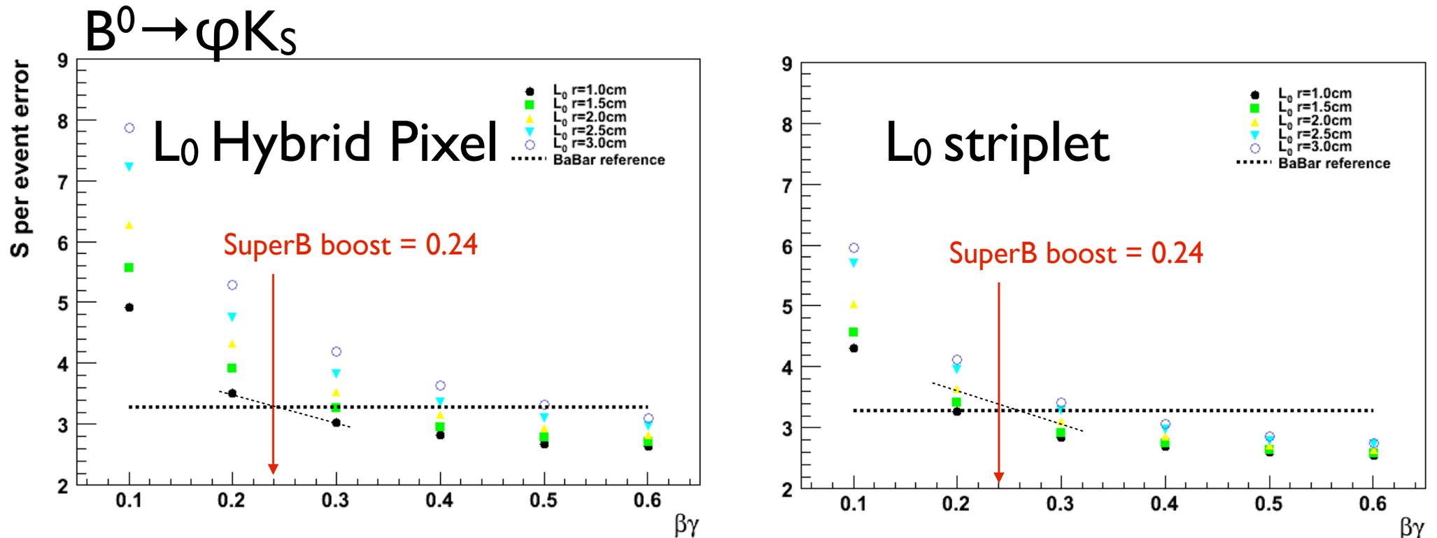
*Hybrid Pixel solution is reaching BaBar reference for  $S$  ( $\sin(2\beta)$ ) per event sensitivity with  $L_0$  radius  $\sim 1.0$  cm. Triplet solution can afford a larger  $L_0$  radius  $\sim 2.0$  cm where bkg is lower.*
