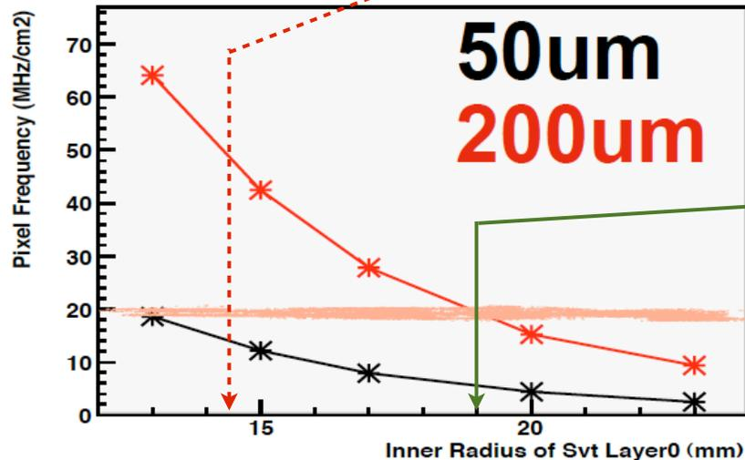
*Triplet solution with  $\langle r \rangle = 1.9$  cm ( $\min(\text{radius}) = 1.7$  cm) seems to satisfy both proper-time resolution and bkg rate requirements.*
