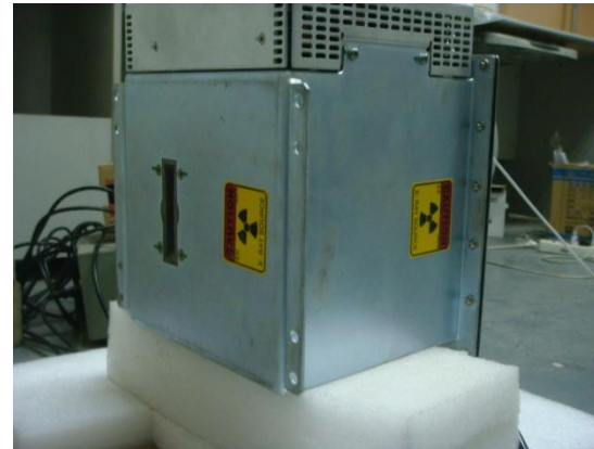
Spellman™ XRB80 High Voltage: 60kV Current: 0.5mA Dose Rate: 2.16 \times 10^{-3} Gy/h (at 1 m)
