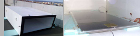
Figure 8: Photos of the thermal amplitude reduction box placed on the building's roof. On the right we can see the test module inside.
