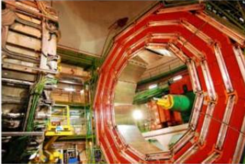
Figure 30: Drift tubes inserted in one of the wheels of CMS. The red part is the iron yoke of the CMS solenoid which houses the muon detectors; in (b) one can see the detector providing a muon measurement extending up to the interaction point with several points (blue) given from the four layers of drift tubes.
