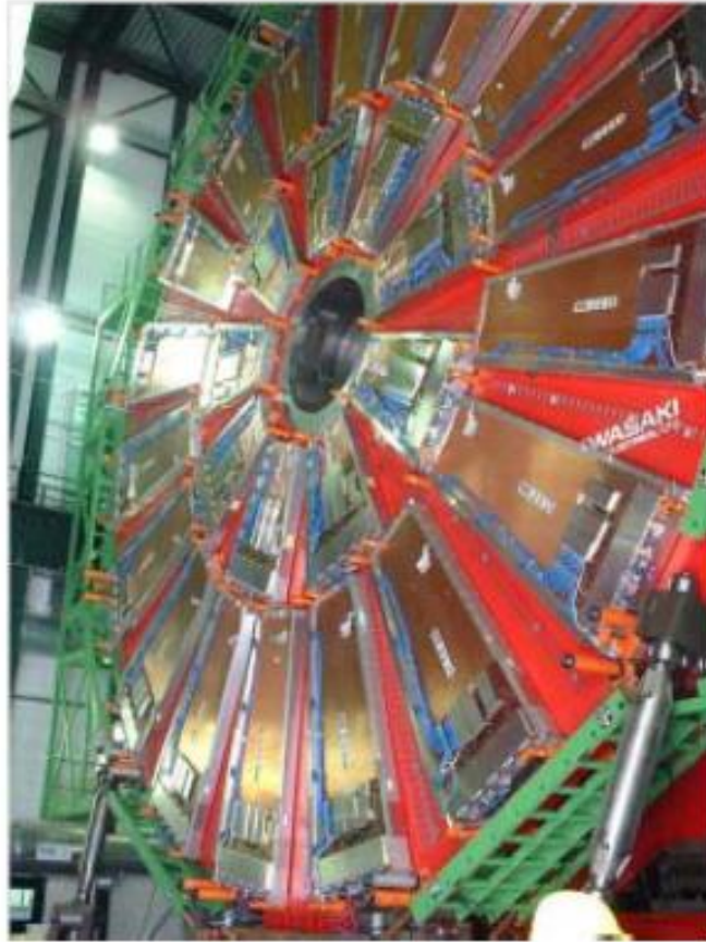
Figure 33: Cathode Strip Chambers mounted on a CMS Endcap
