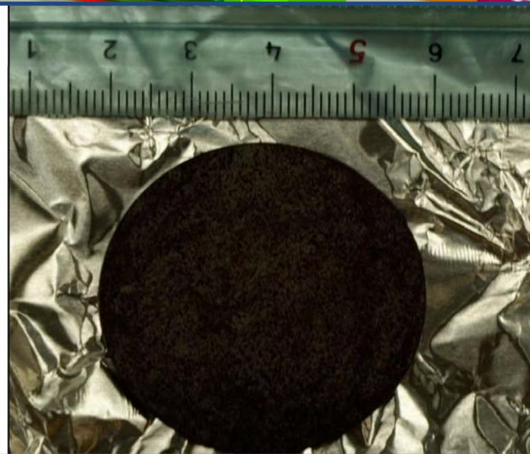
UCx pellets production: 1 mm thick, 40 mm dia
