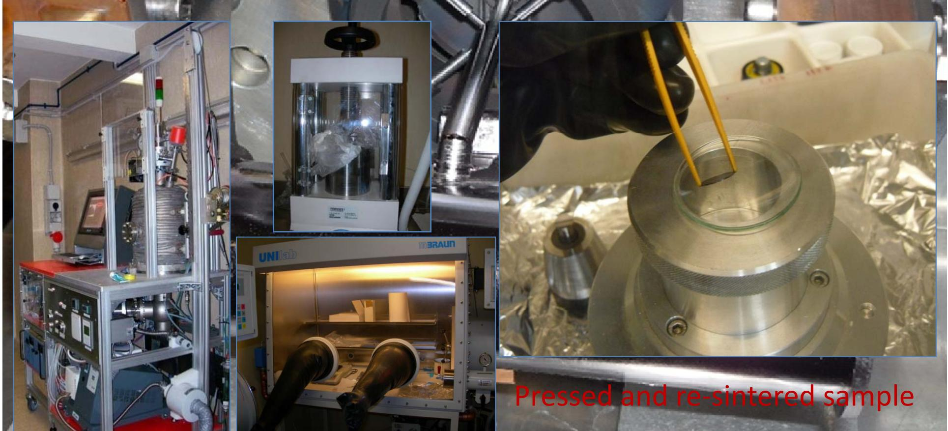
Pressed and re-sintered sample
