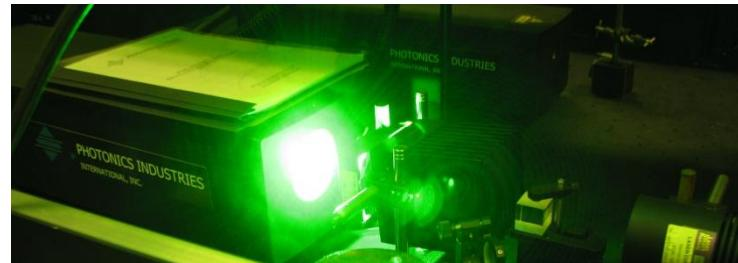
Pump laser: Nd:YAG (532 nm),
