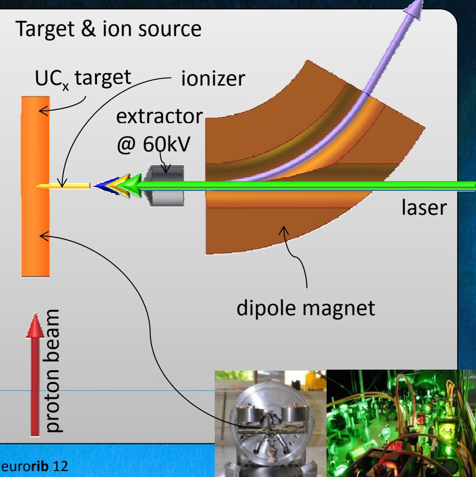
Resonance ionization laser ion source (RILIS)
