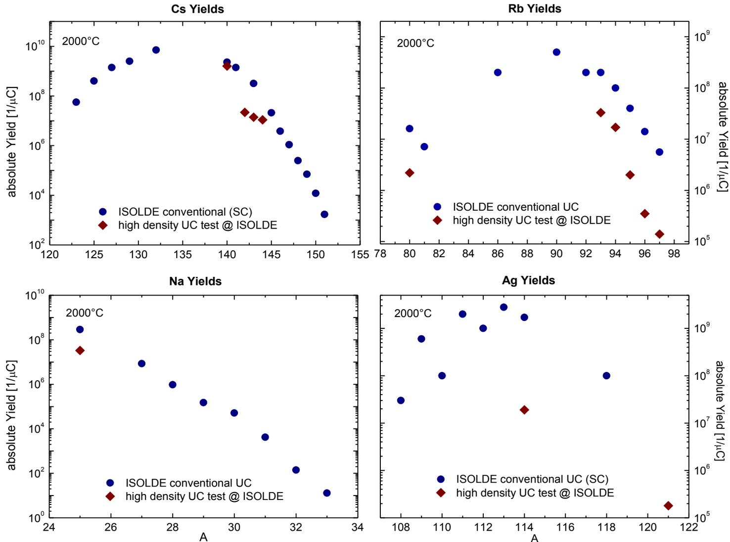
HD absolute yields @ ISOLDE (450g) x2 to x10 lower than from conventional UC targets (~100g)
