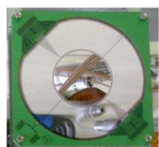
Annular Si (500 $\mu\text{m}$  thick)
