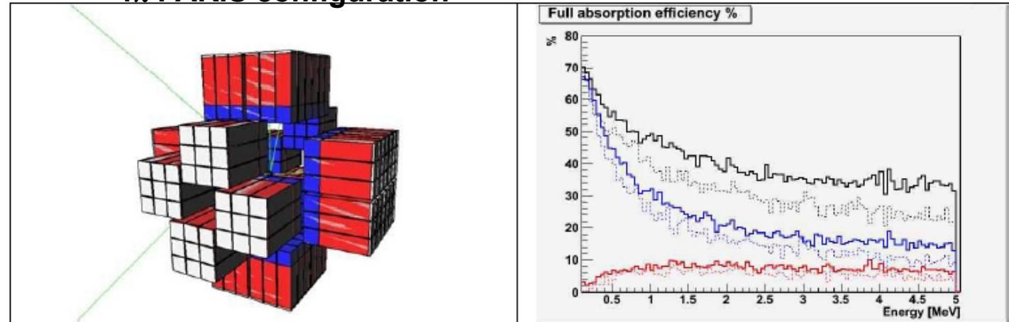
Efficiency gain of a factor  $\sim 20$  for p- $\gamma$  coincidences for  $^{132}\text{Sn}(\text{d},\text{p})$  @ 10 MeV/u
