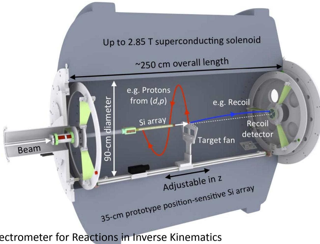
A Solenoid Spectrometer for Reactions in Inverse Kinematics
