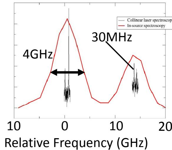
**Combining high resolution nature of collinear beams method with high sensitivity of in-source spectroscopy. Allowing extraction of B factors and quadrupole moments.**
