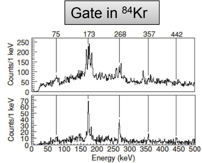
FIG. 3. Spectrum of  $\gamma$ -ray energies from targetlike fragments gated on the beamlike fragments  $^{84}\text{Kr}$  (top) and on beamlike fragments  $^{84}\text{Kr}$  plus a short time of flight (bottom). The transitions identified as the rotational band in  $^{168}\text{Dy}$  are marked with solid lines.
