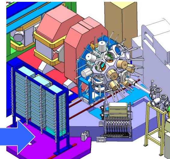
AGATA is a last generation gamma spectrometer built to serve the most demanding needs of present and future Radioactive Ion Beam (RIB) facilities.
