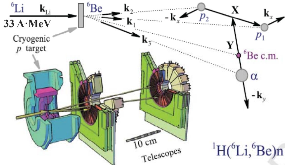
Experimental setup and kinematical diagram. ↑↑
