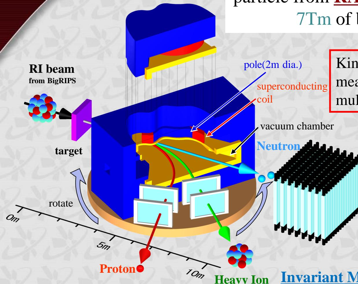
Kinematically complete measurements by detecting multiple particles in coincidence
