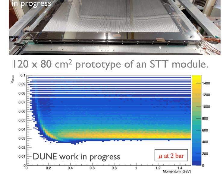
Measured prototype dE/dx resolution
