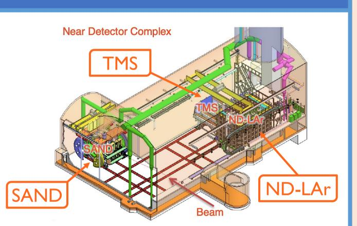
SAND will stand at a fixed position along the beam axis, while ND-LAr and TMS will be movable off-axis, for datataking in different energy intervals.
