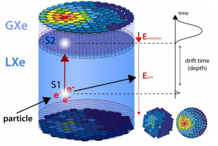
Schematic of the working principle of a dual-phase time projection chamber (TPC).
