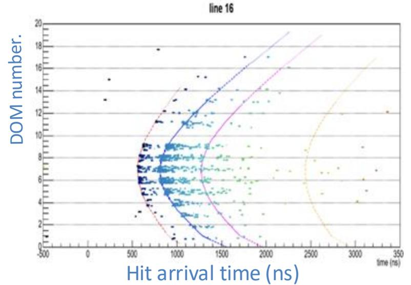
Hit times fully consistent with photons from Cherenkov emission
