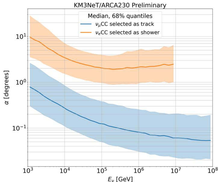
Time Synchronisation and DOM position calibration is the key parameter to optimise angular resolution
