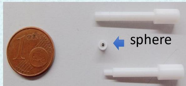
Spheres are free to rotate for correct alignment (easy axis || B)
