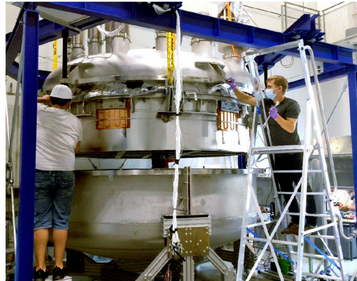
Test electrodes with 2.6 m \varnothing
