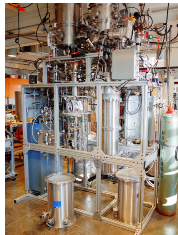
Example: Xeclipse, a xenon purification system at Columbia University (demonstrator for XENONnT at LNGS), Plante, Aprile, Howlett, Zhang, arXiv:2205.07336
