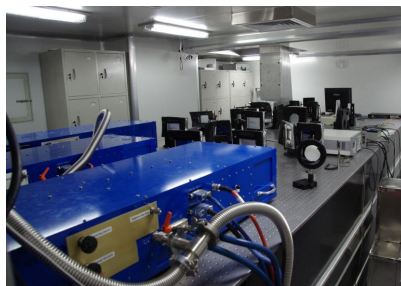
CO 2 -pumped HCOOH lasers (0.694THz)
