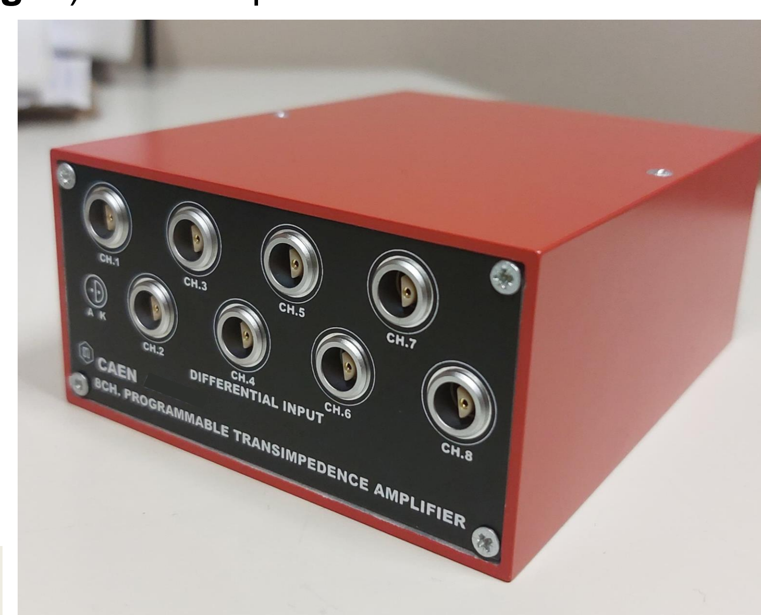
Figure 4: The new 8-channel low-noise current amplifier prototype developed by CAEN.
