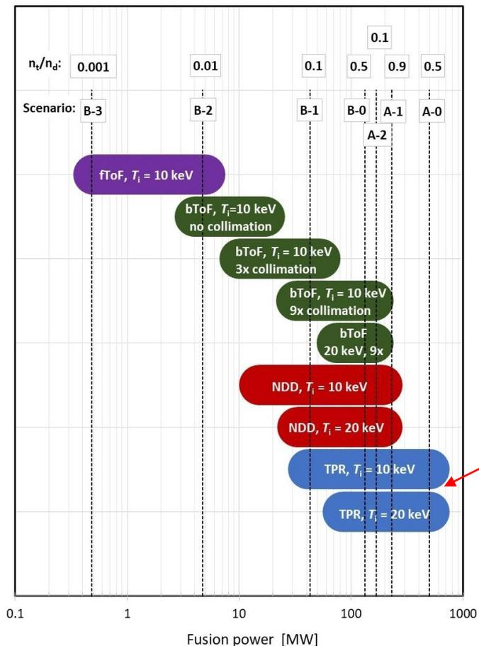
To fulfill the requirement on  $n_T/n_D$  for a fusion power range of 0.5 to 500 MW, four different neutron spectrometers are proposed. The set of neutron spectrometers suggested for the HRNS system are as follows:
