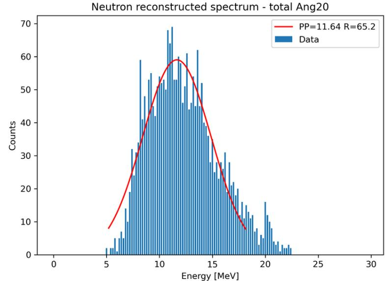
**Issue of energy reconstruction (energy shift)** – likely related to readout electronics (crosstalk between the readout planes), but it needs to be studied further
