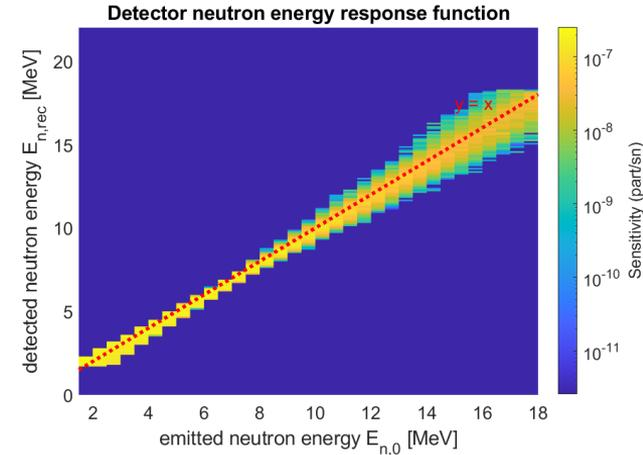
→ Energy resolution can be increased at the cost of efficiency (decreased count rate)
