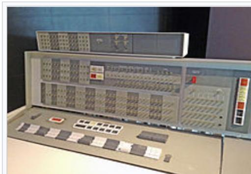
IBM 7094 operator's console showing additional index register displays in a distinctive extra box on top. Note "Multiple Tag Mode" light in the top center.
