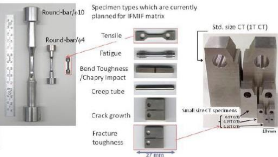
Samples and irradiation modules developed for the IFMIF facility
