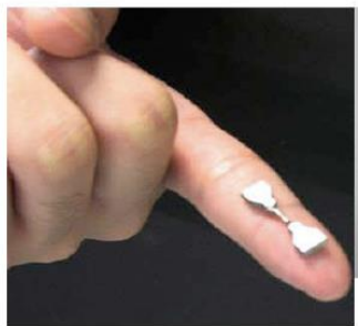
Samples and irradiation modules developed for the IFMIF facility
