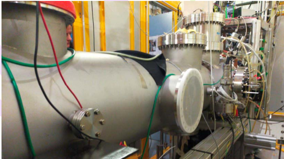
NIO1: a beamline view (with the source in the background); note open flanges, from which pumps were removed (we may worry for cesium oven oxidation; we will probably learn something)
