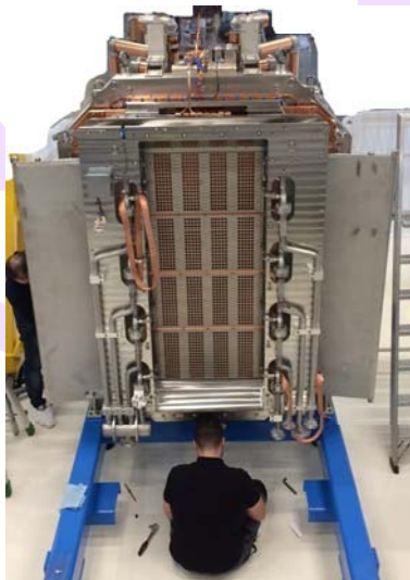
Front view of SPIDER, note Grounded Grid
